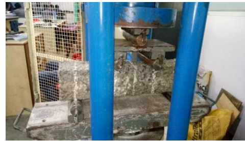
Figure h: Flexural test (with fibre)
