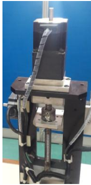
Figure 4: The spiral rod for upward-downward movement of the mechanical arm for lifting the standard weight up in the weight scale calibration
