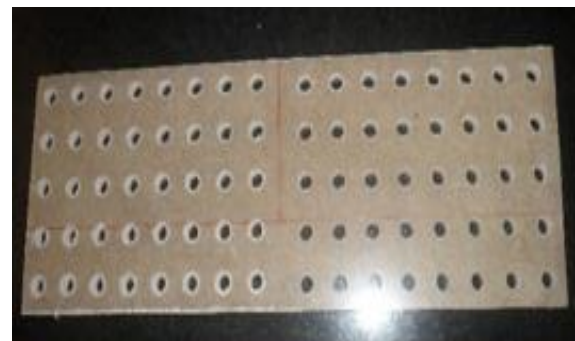
Figure 3: Holes drilled on the work piece for each experimental run
