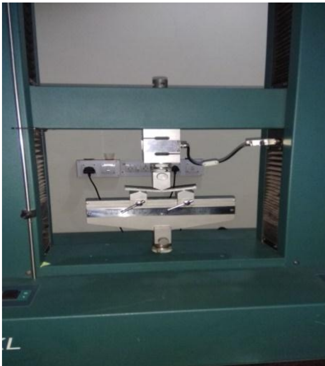
Figure 4 Experimental setup for flexural testing
