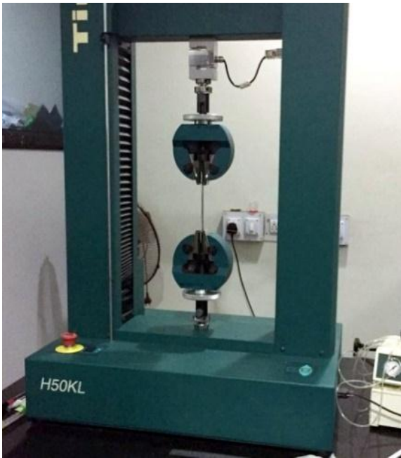
Figure 3 Experimental setup for tensile testing
