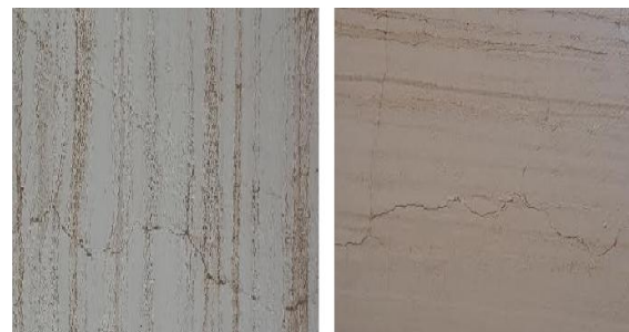
Figure 13. Contraction test by addition of fibre
