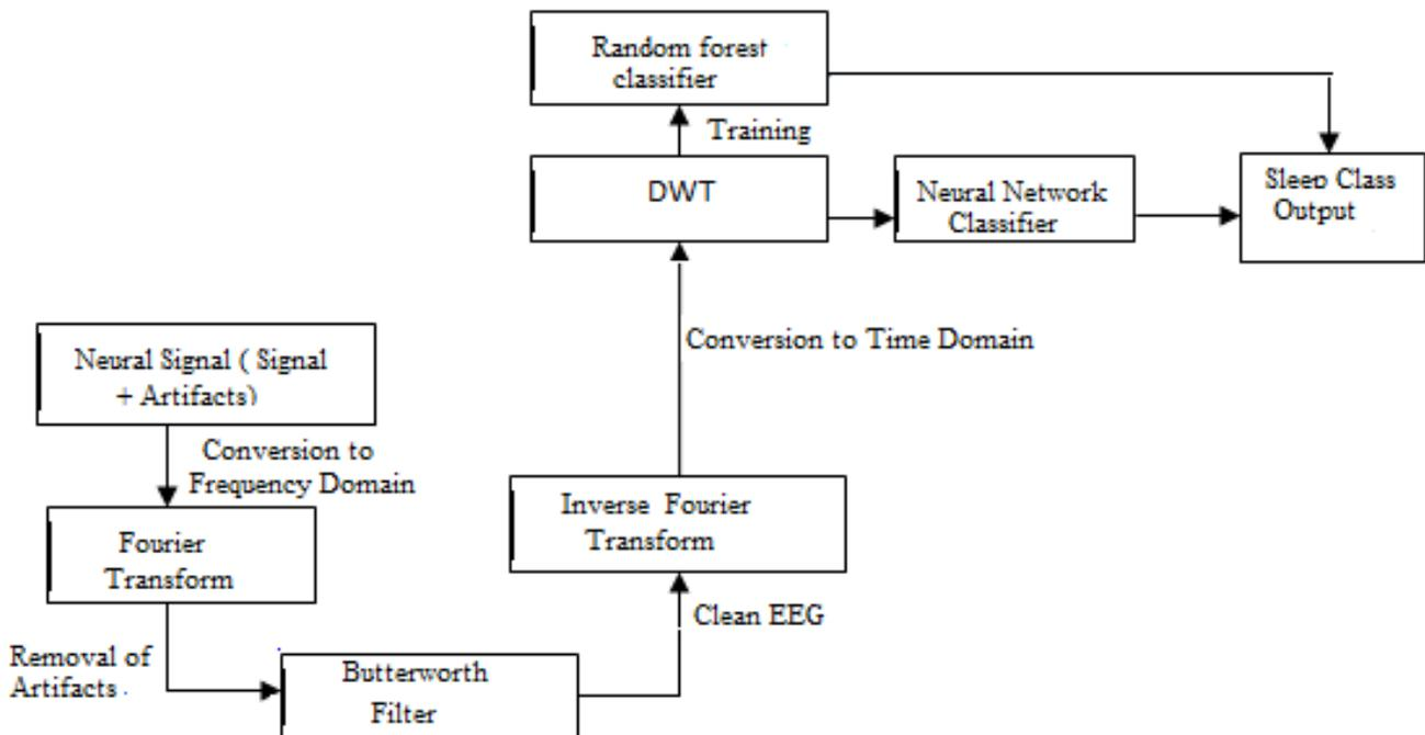
Figure 2. Architecture for Detection of Sleepiness
