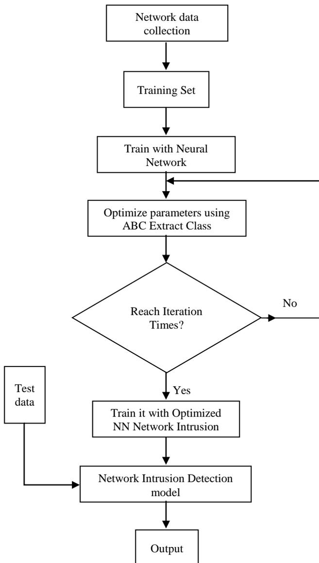
**Figure 4:** Flow diagram for ABC-BP Neural Network based network intrusion detection model
