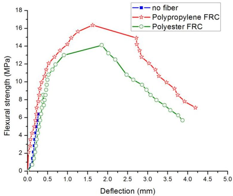
**Figure 4.** Variation of flexural strength with deflection of ECC mixes
