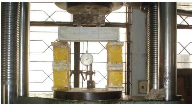
**Figure 2.** Flexural Test setup
