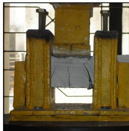
**Figure 5.** Double shear Test setup
