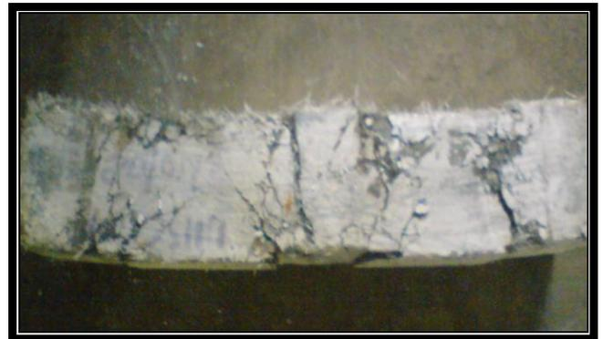
a) Failure pattern of Polypropylene ECC beam
