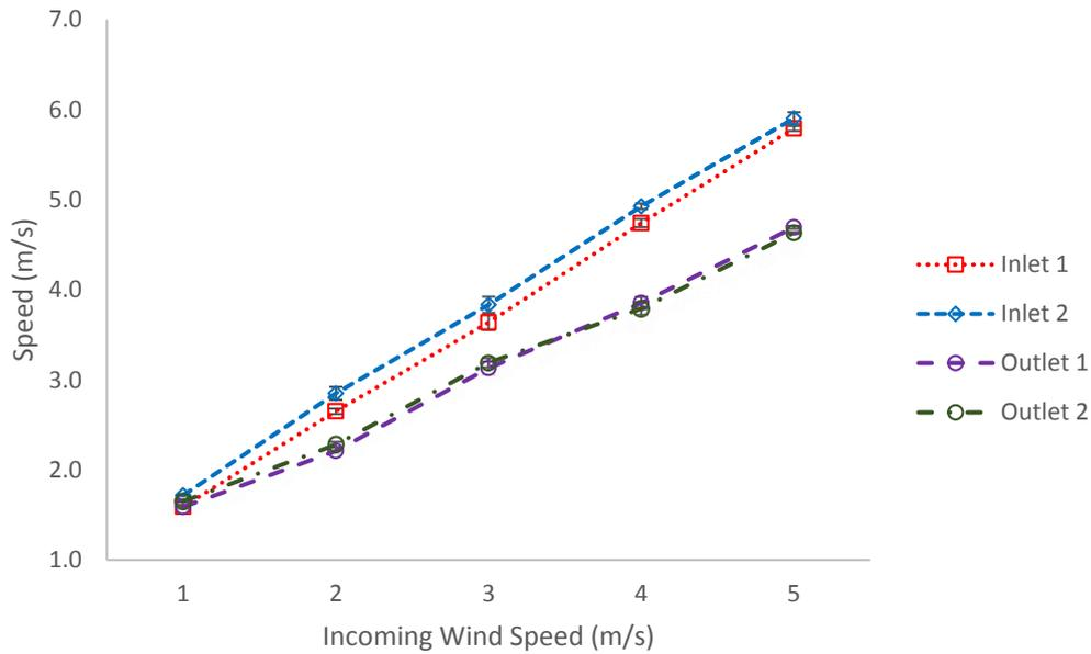
**Figure 8.** Comparison of speed at various openings near the flat surface roof with incoming wind speeds of 1-5 m/s from south direction
