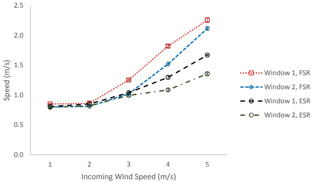
**Figure 14.** Comparison of speed at window openings 1 and 2 for flat surface roof (FSR) and ellipse surface roof (ESR) with incoming wind speeds of 1-5 m/s from south direction
