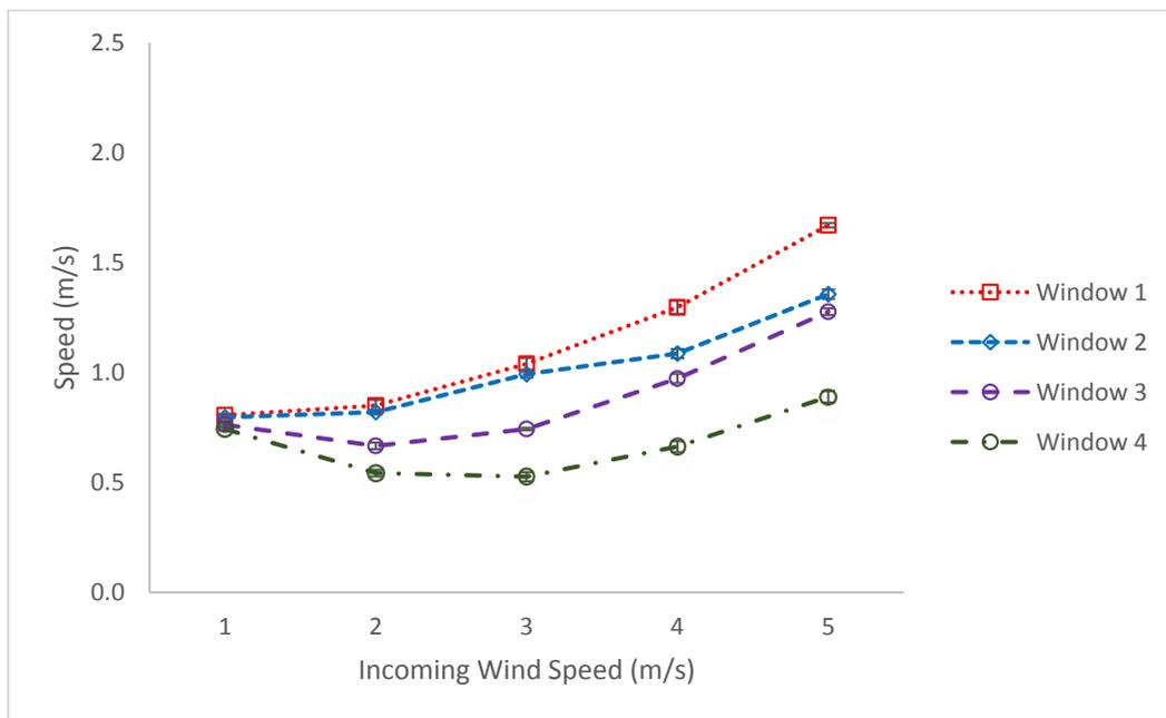
**Figure 13.** Comparison of speed at window openings for ellipse surface roof with incoming wind speeds of 1-5 m/s from south direction
