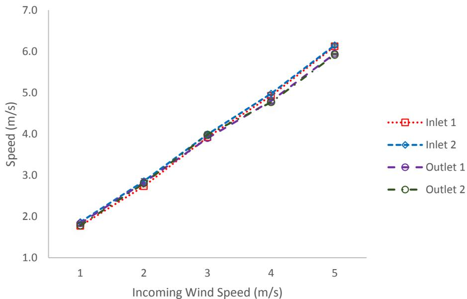
**Figure 9.** Comparison of speed at various openings near the ellipse surface roof with incoming wind speeds of 1-5 m/s from south direction
