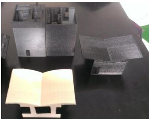
**Figure 3.** Model of 1:50 scaled flat and ellipse roof and the joined stair and wall part
