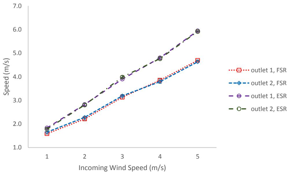
**Figure 11.** Comparison of speed at outlets near the flat surface roof (FSR) and ellipse surface roof (ESR) with incoming wind speeds of 1-5 m/s from south direction
