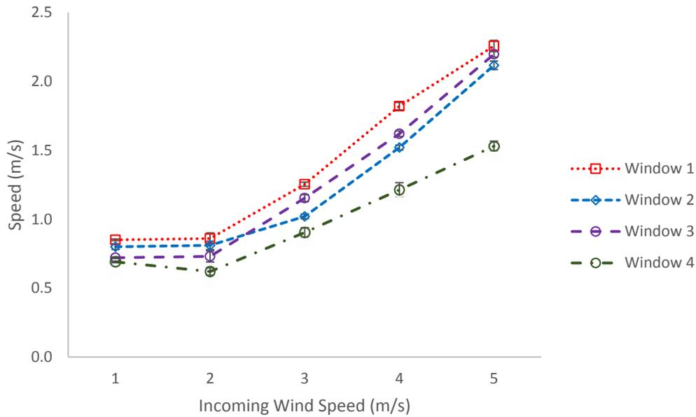
**Figure 12.** Comparison of speed at window openings for flat surface roof with incoming wind speeds of 1-5 m/s from south direction
