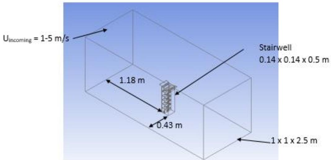
**Figure 5.** Illustration of experimental setup in wind tunnel test section
