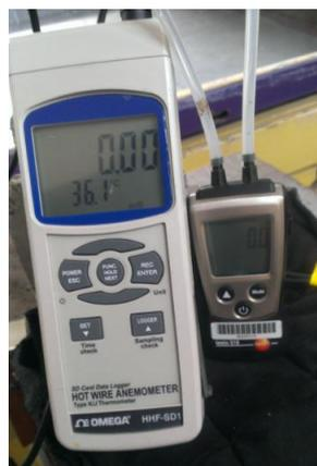
(b) Display of anemometer (air temperature in °C and air velocity in m/s) and display of Testo 510 for the pitot-tube
