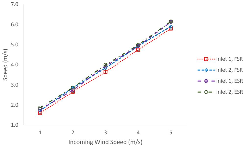
**Figure 10.** Comparison of speed at inlets near the flat surface roof (FSR) and ellipse surface roof (ESR) with incoming wind speeds of 1-5 m/s from south direction
