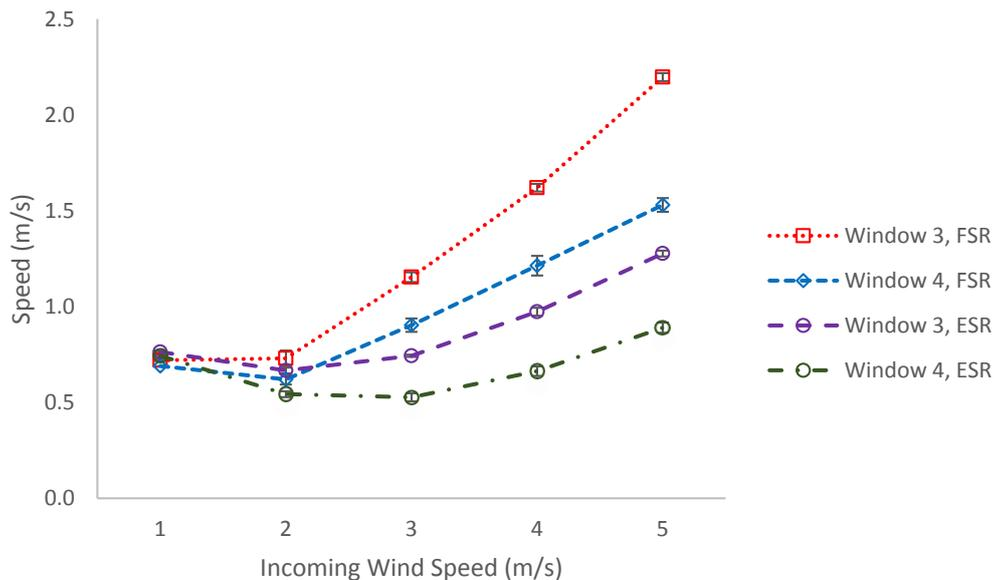
**Figure 15.** Comparison of speed at window openings 3 and 4 for flat surface roof (FSR) and ellipse surface roof (ESR) with incoming wind speeds of 1-5 m/s from south direction
