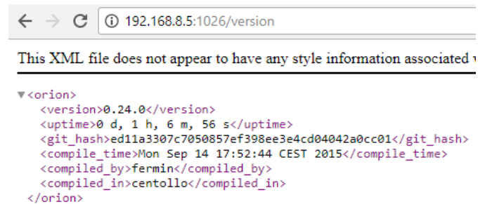
Figure 6: Confirmation of the execution of the Orion Context Broker.
