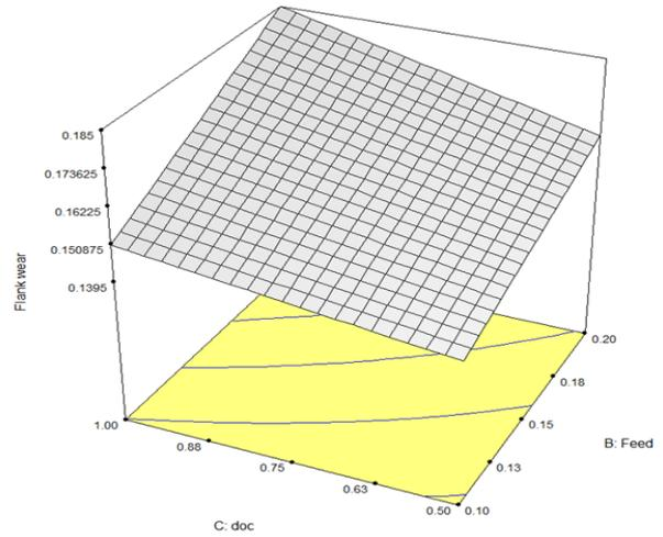
**Figure 4:** Flank wear of carbide tools depending on feed rate and depth of cut
