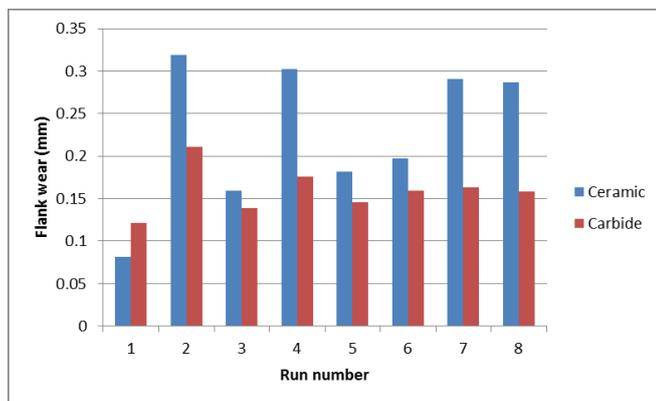
**Figure 7:** Comparison of flank wear between ceramic and tungsten carbide tools.
