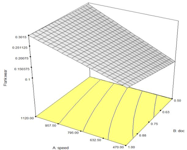
**Figure 5:** Flank wear of ceramic tools depending on cutting speed and depth of cut
