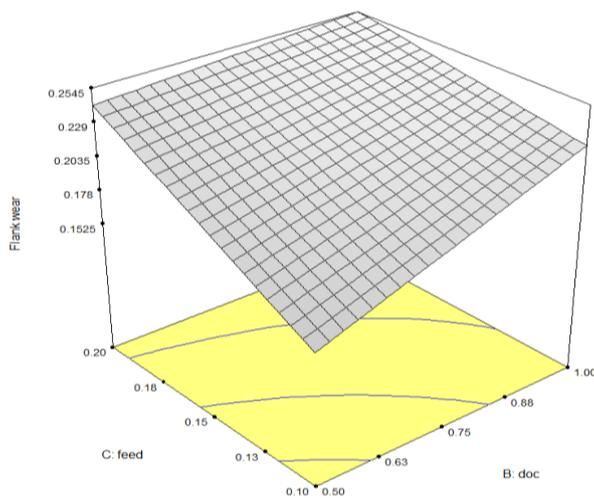
**Figure 6:** Flank wear of ceramic tools depending on feed rate and depth of cut
