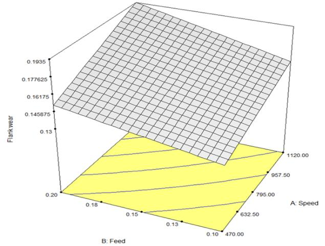
**Figure 3:** Flank wear of carbide tools depending on cutting speed and feed rate
