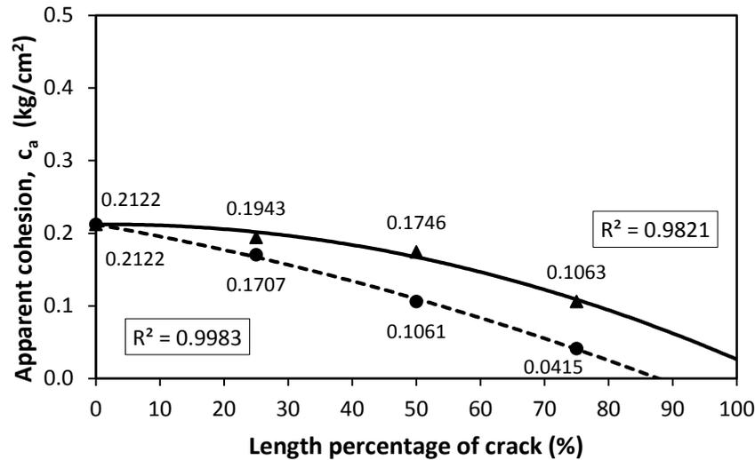
Figure 4. Apparent cohesion on crack plane in soil
