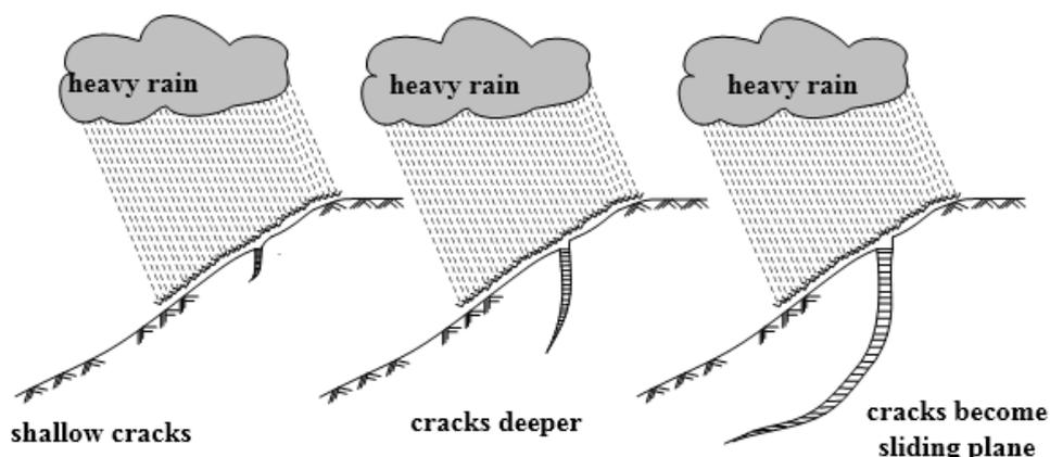
Figure 1. Cracks propagation on heavy rain
