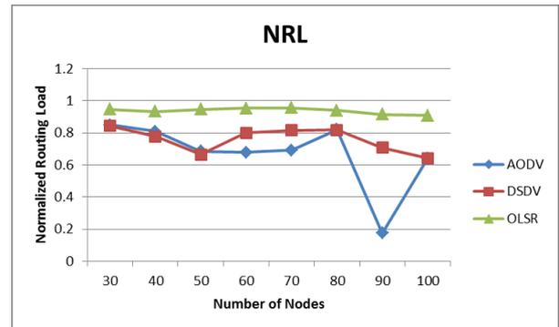
Figure 6: Normalized routing load
