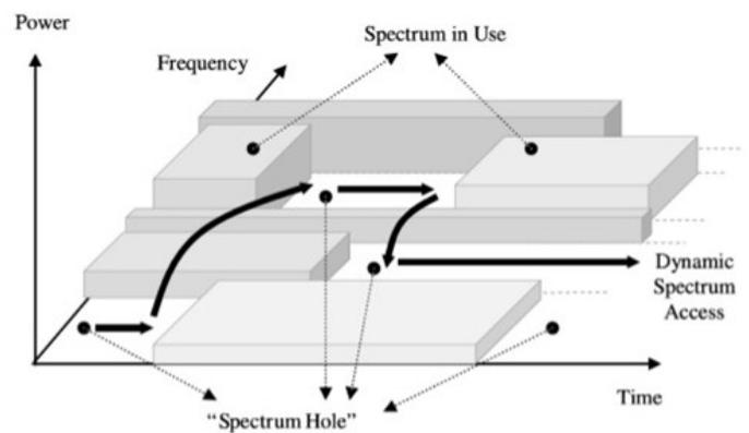
Figure 2: Spectrum hole concept [7]
