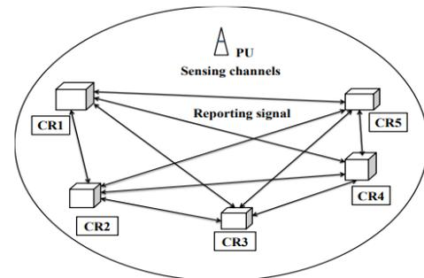
Figure 6: Distributed sensing [103]
