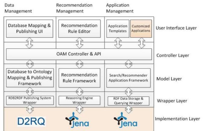
Figure 3: Layered architecture of the OAM framework [14]
