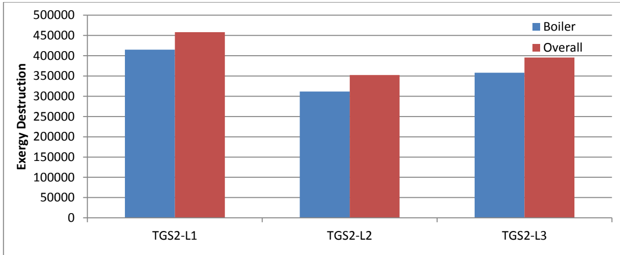
Figure 12. Exergy Destruction of Turbo-Generator Set-2 at Various Operating Loads
