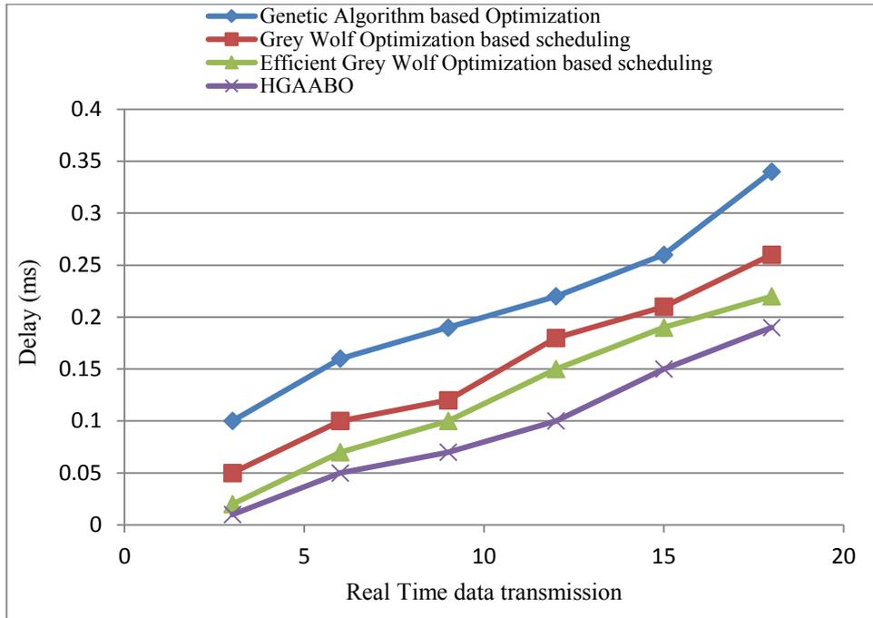
**Figure. 9:** Delay with Respect to Real Time Data Transmissions
