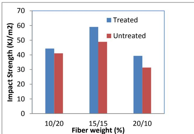
**Figure 3.** Variation of maximum Impact Strength with ratio of Prosopis Juliflora/glass reinforced Epoxy Composites for treated and untreated composites
