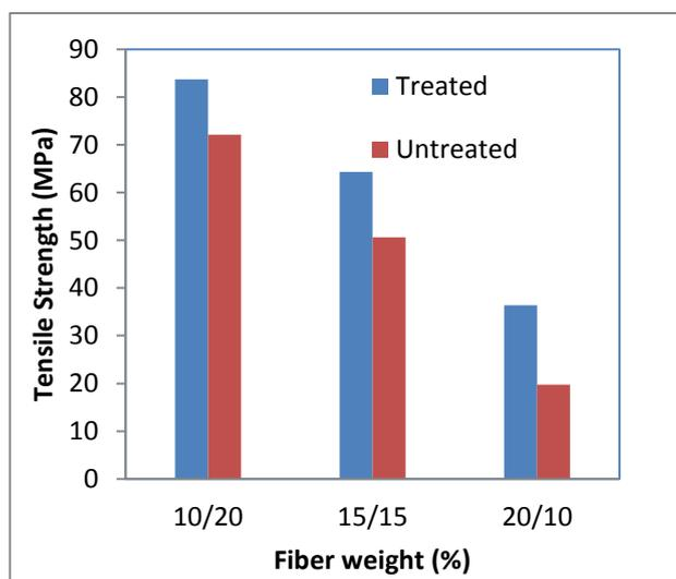
**Figure 1.** Variation of maximum Tensile strength with ratio of Prosopis Juliflora/glass reinforced Epoxy Composites for treated and untreated composites
