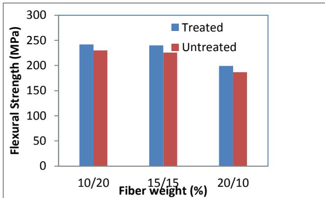
**Figure 2.** Variation of maximum Flexural Strength with ratio of Prosopis Juliflora/glass reinforced Epoxy Composites for treated and untreated composites
