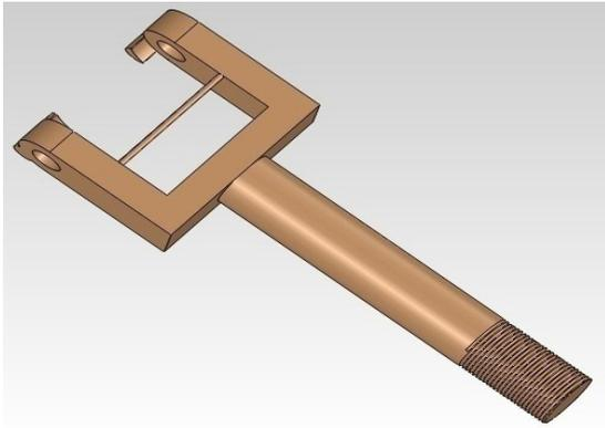
**Figure 9:** 3D views of supporting cum limiting rod (new fixture)
