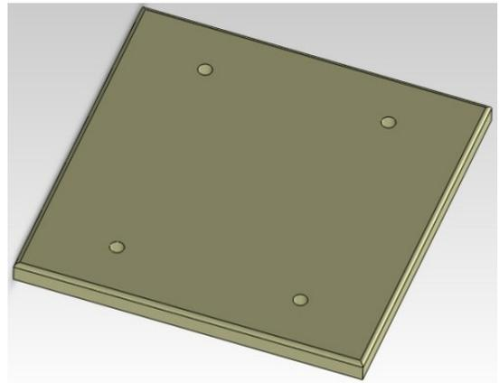
Figure 7: 3D view of fixture bed (new fixture)
