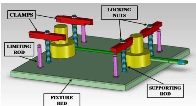
Figure 5: 3D view of present fixture
