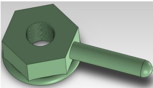
**Figure 10:** 3D view of locking nut (new fixture)
