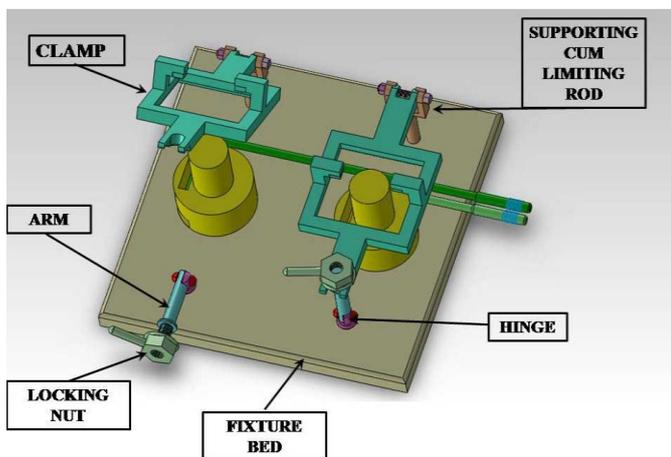
Figure 6: 3D view of new fixture
