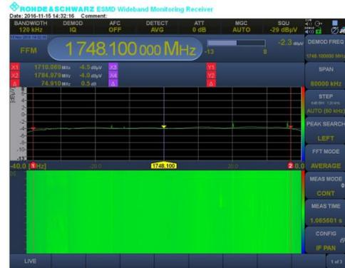
**Figure 8:** Spectral occupancy of the 1800 MHz band -Uplink
