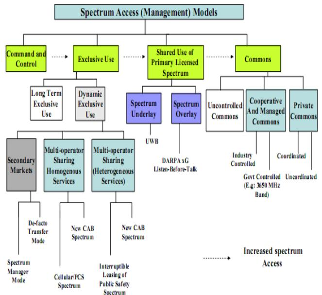
Figure1: Classification of spectrum access models [4]
