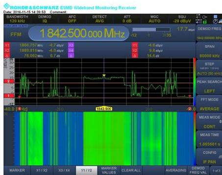
**Figure 7:** Spectral occupancy of the 1800 MHz band - Downlink
