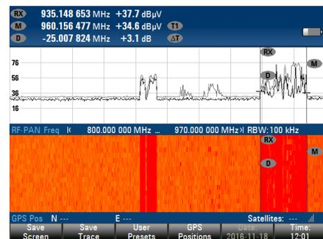
**Figure 5:** Spectral occupancy of the 900 MHz Band
