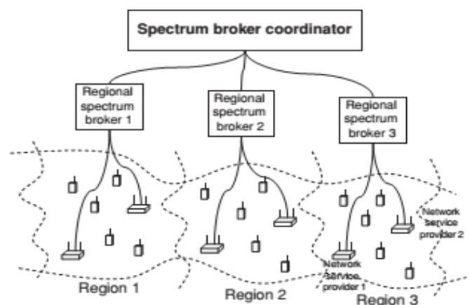
**Figure 2:** Spatio-temporal dynamic spectrum access model [1]
