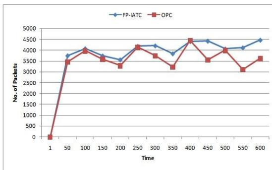
**Figure 5:** Packet loss comparison of OPC with FP-IATC
