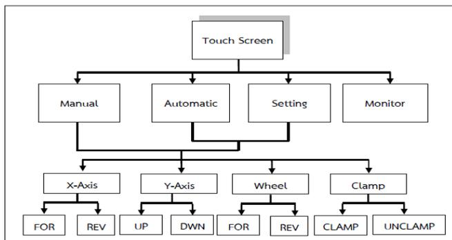
**Figure 6:** The instruction diagram of the touch screen monitor
