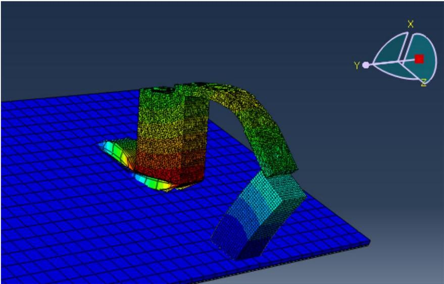
**Figure 10:** First elastic mode of suggested model ( $f_n = 2.18$ ).
