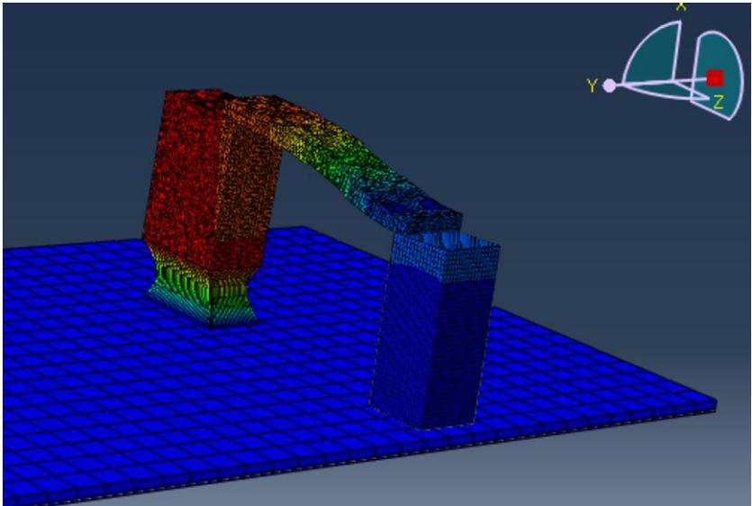
**Figure 11:** Second elastic mode of suggested model ( $f_n = 2.45$ ).
