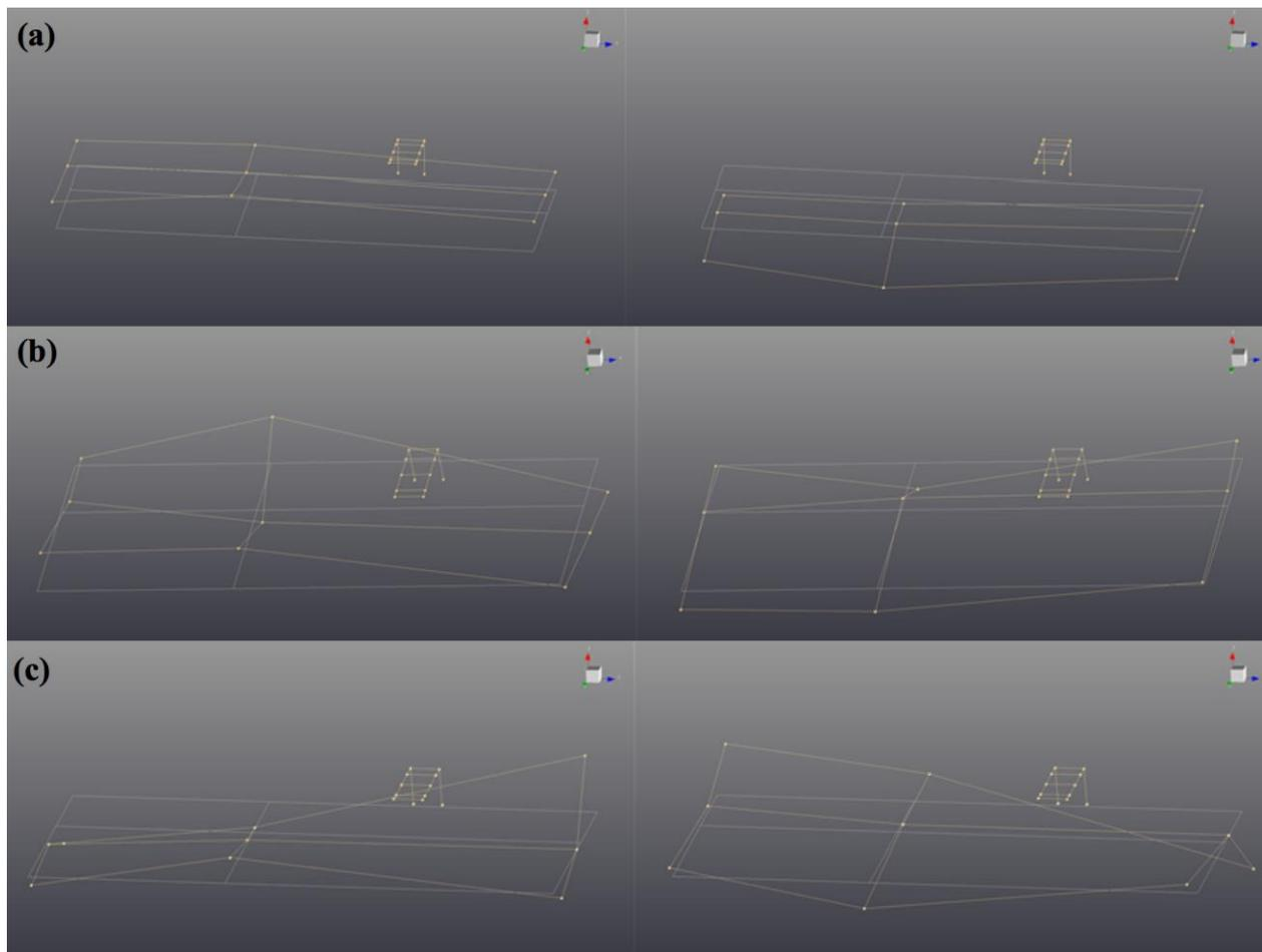
**Figure 12:** Experimental modes of plate, (a) rigid body mode  $f_n = 0.78$ , (b) bending mode  $f_n = 1.2$ , and (c) torsional mode  $f_n = 2.7$ .
