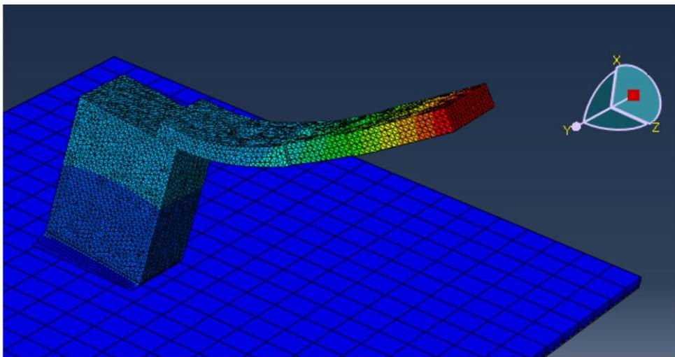
**Figure 7:** Correlated results (first bending mode,  $f_n = 0.92$ ).
