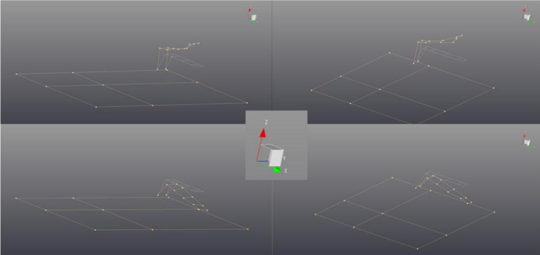
**Figure 3:** Measured mode that rotates around y-axis ( $f_n = 0.45$ ).
