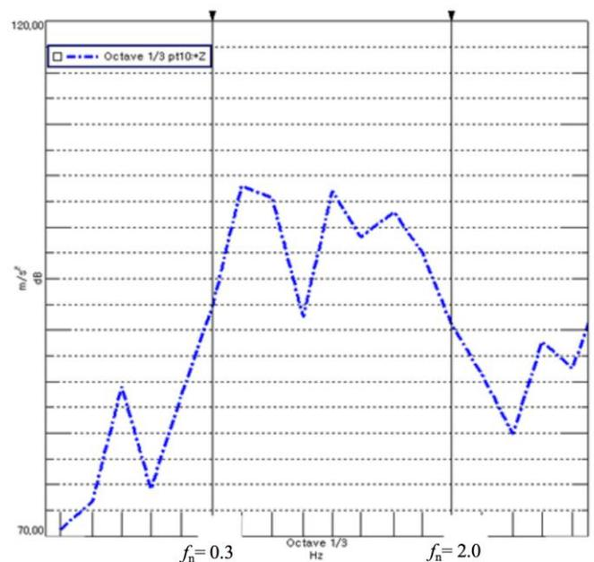
**Figure 8:** Input vibration close to the motor.
