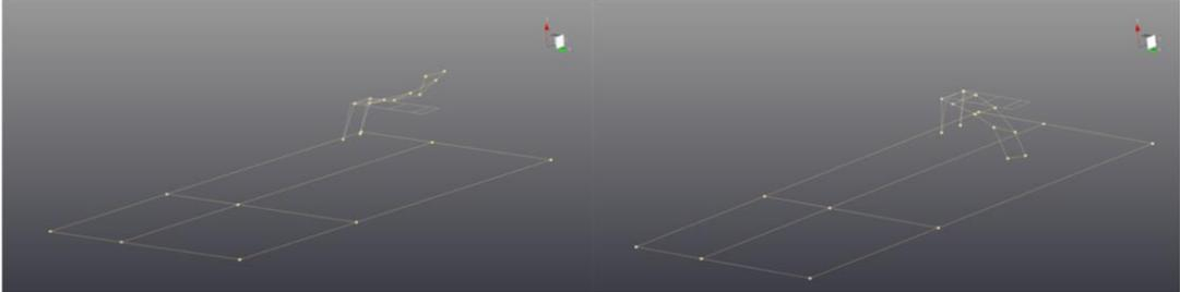
**Figure 4:** Measured first bending mode ( $f_n = 0.90$ ).
