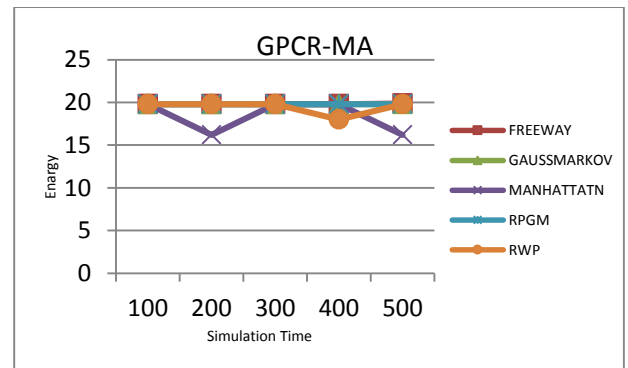
Figure 4: Comparison of the Energy consumption between Freeway, Gauss-Markov, Manhattan, RPGM and RWP Mobility Model based on the simulation time using GPCR-MA protocol.
