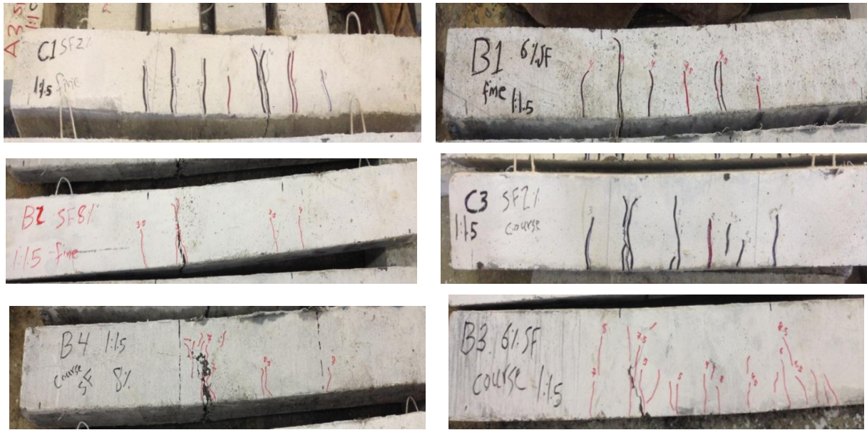
Figure 14: Cracking of failure specimens for group 2 (C1, C3, B1, B2, B3 and B4)
