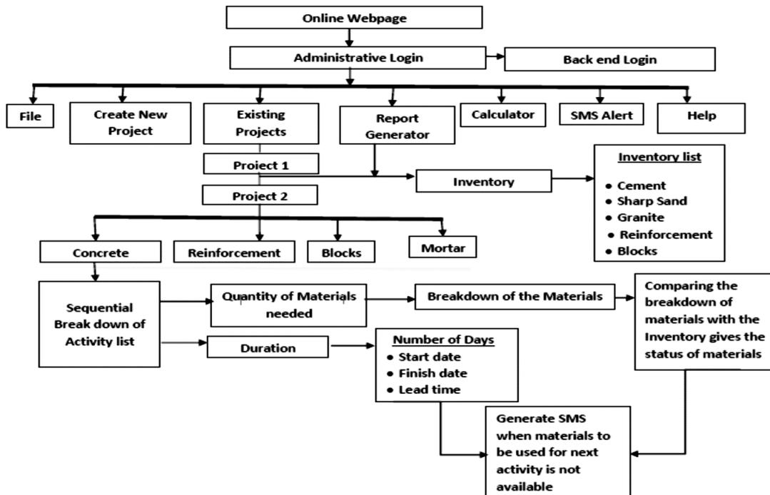
Figure 4. System Block Diagram of the WB-MPC
