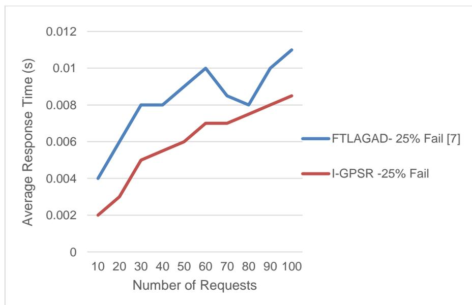
Figure 1: Average Response Time with 25% Failure of Vehicles
