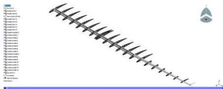
Figure 5. Prototype wing structure Source: Own work
