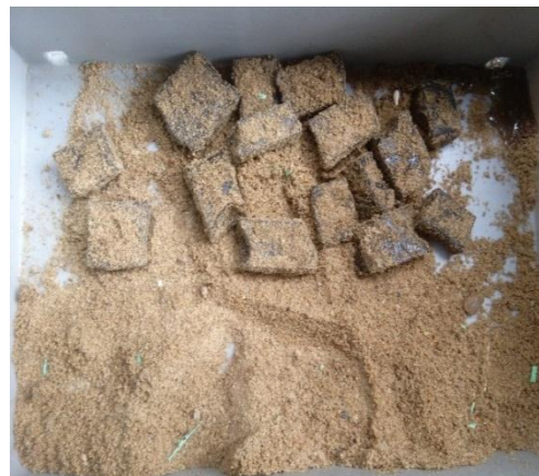
Fig.4 Combining Sand and Rubber Shreds (with resin)
