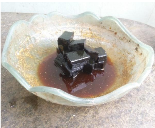
Fig.3 Mixing of Rubber Shreds with Resin
