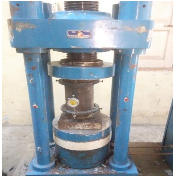
Fig.11 Test Set-up for Cylinder Specimen
