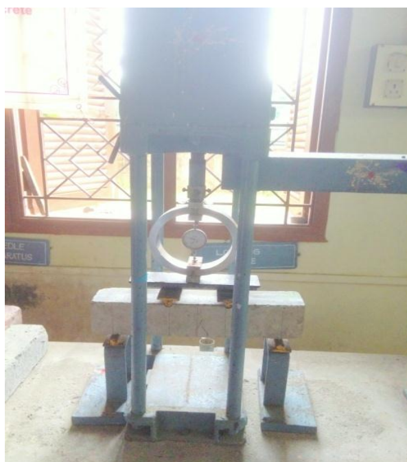
Fig.9 Test Set-up for Prism Specimen
