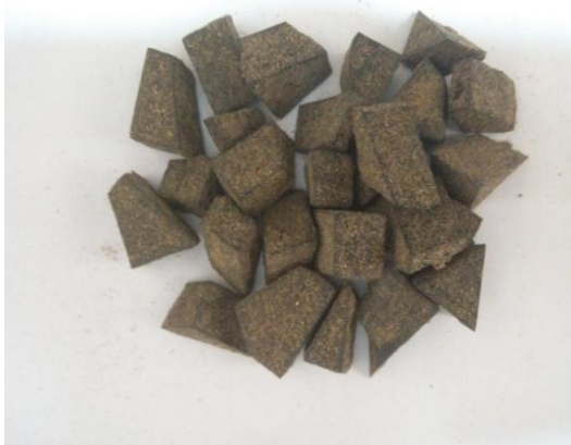
Fig.5 Sand Coated Rubber Shreds
