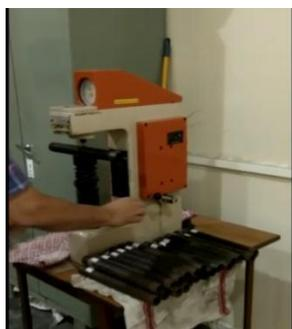
**Figure 2.** Hardness test set-up
