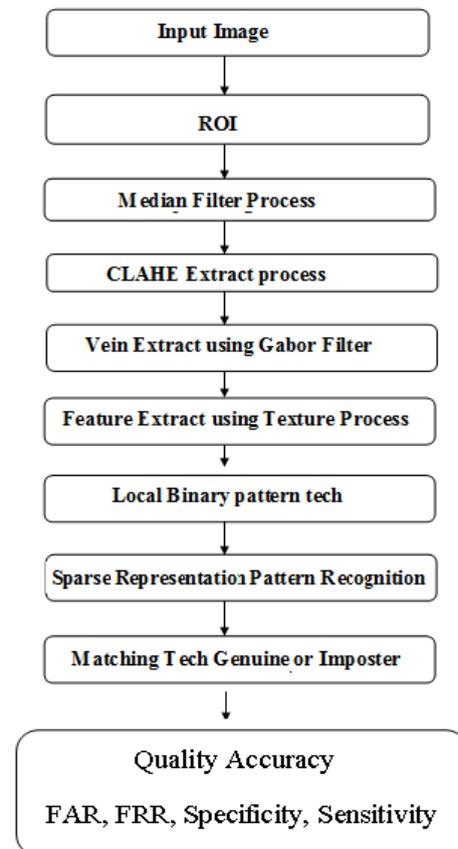
Fig. 1. Typical Process of finger vein identification
