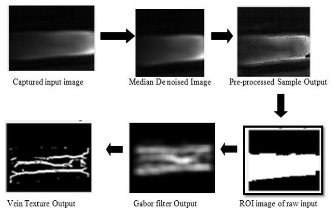
**Fig 3:** Process of Finger vein images
