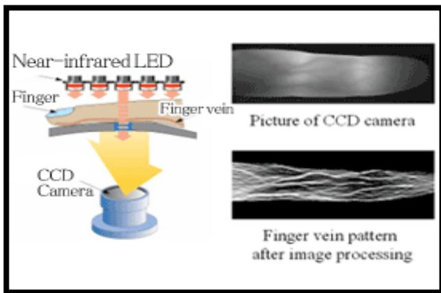
**Fig. 2.** Capturing Finger Vein pattern using CCD Camera
