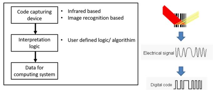
**Figure 4:** Working of One Dimensional or linear code Data Capturing Technique
