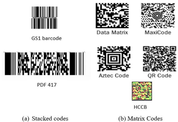
**Figure 7:** Examples of stacked and matrix codes
