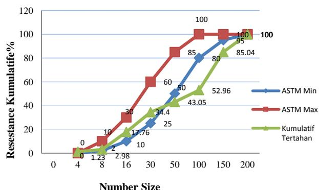
**Figure.2** The results of sieve test of fine aggregates of Pohara sand
