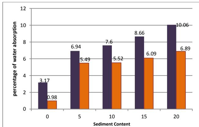
Figure 3.a and b The Results of Compressive Strength and Water Absorption Tests using a ratio 1 : 3 of Cement and Sand
