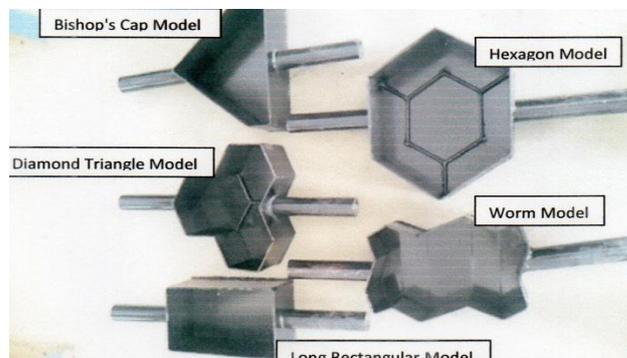
**Figure 1.** Paving block molds
