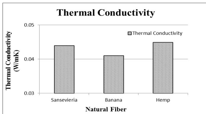
Figure 6: Effect of fiber on Thermal Conductivity
