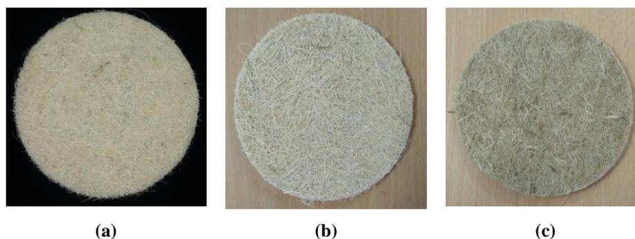
**Figure 2:** Needle punched Nonwoven fabrics (100%)
