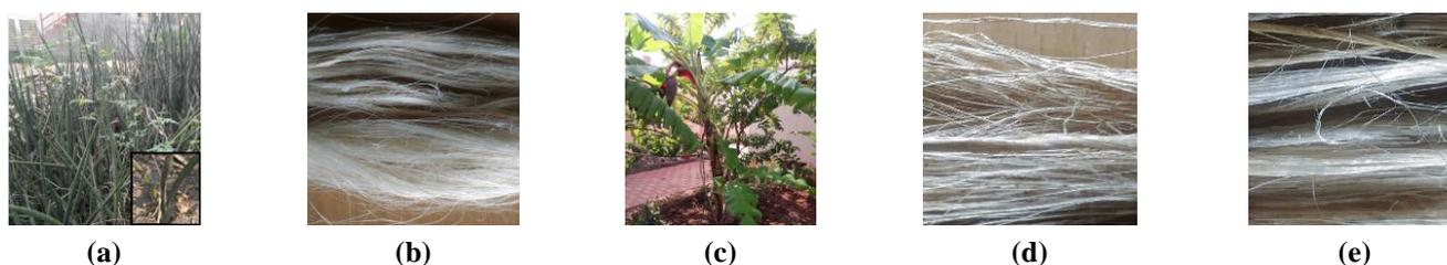
**Figure 1:** (a) Sansevieria stuckyi plants (b) Sansevieria stuckyi fibers (c) Banana pseudo stem (d) Banana fibers (e) Hemp fibers
