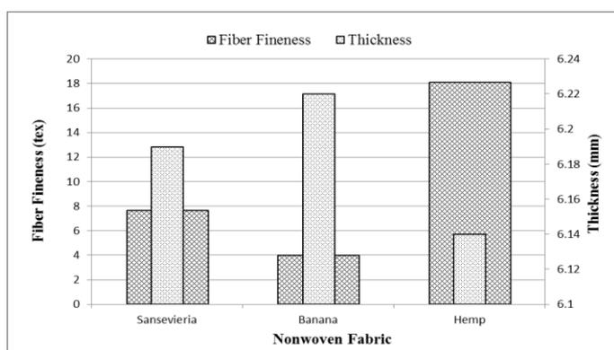
Figure 4: Effect of Natural fibers fineness on thickness of fabric
