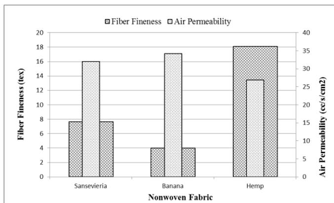
Figure 5: Effect of Natural fibers fineness on Air Permeability of the fabric
