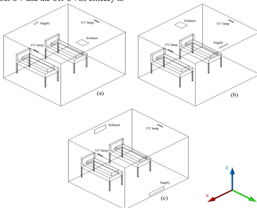
**Figure 1.** Schematic of the patient room with (a) mixing ventilation, (b) downward ventilation, and (c) displacement ventilation
