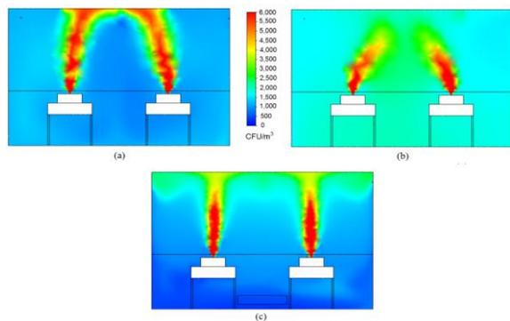
**Figure 3.** *S.aureus* distribution without UVGI on sampling plane (x-z) for (a) mixing ventilation, (b) downward ventilation, and (c) displacement ventilation
