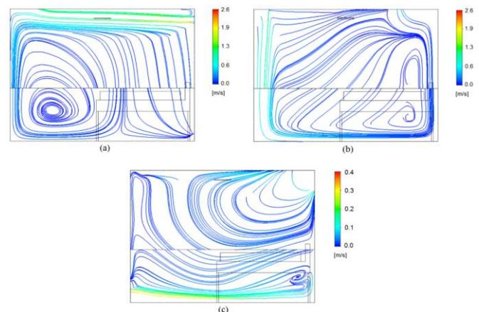
**Figure 2.** Air flow patterns in the room with (a) mixing ventilation, (b) downward ventilation, and (c) displacement ventilation
