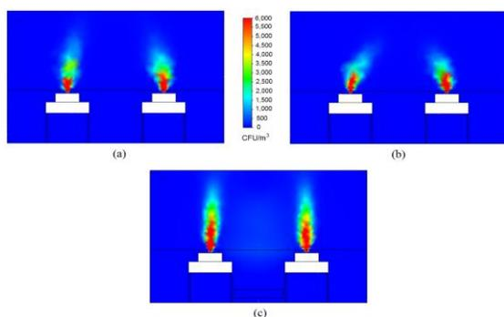
**Figure 4.** *S.aureus* distribution with UVGI on sampling plane (x-z) for (a) mixing ventilation, (b) downward ventilation, and (c) displacement ventilation
