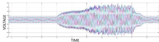
**Figure 9.** Grid voltage curve without battery
