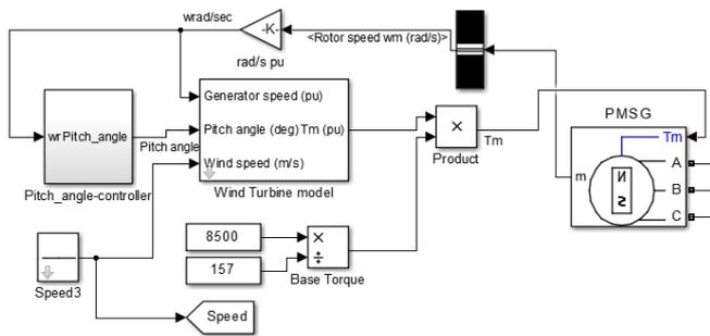
**Figure 1.** Matlab Simulink model of PMSG based wind power generation.
