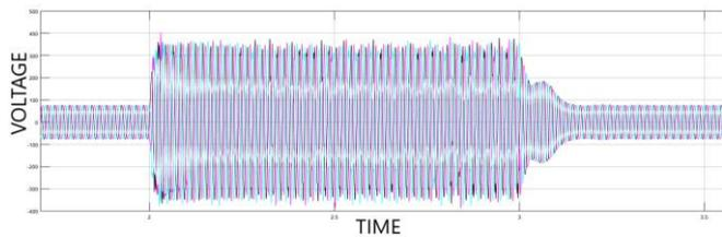
**Figure 15.** Grid voltage curve with battery
