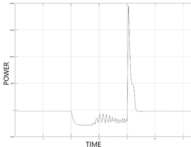
**Figure 11.** Grid power curve without battery
