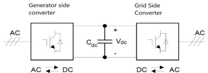
**Figure 3.** Block diagram of back-to-back converters
