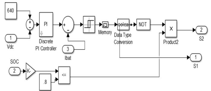
**Figure 5.** Matlab Simulink model of battery controller
