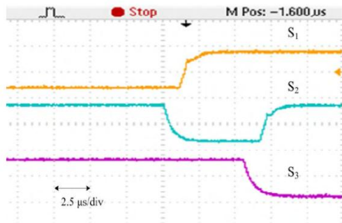
Diagram 12. Gate pulses of one leg of NSC (20V/div) with 1_μs dead band.
