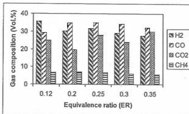
Figure 6. Influence of equivalence ratio on gas composition volume %
