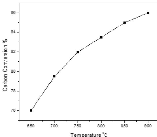
Figure 5. Influence of temperature on Carbon conversion efficiency
