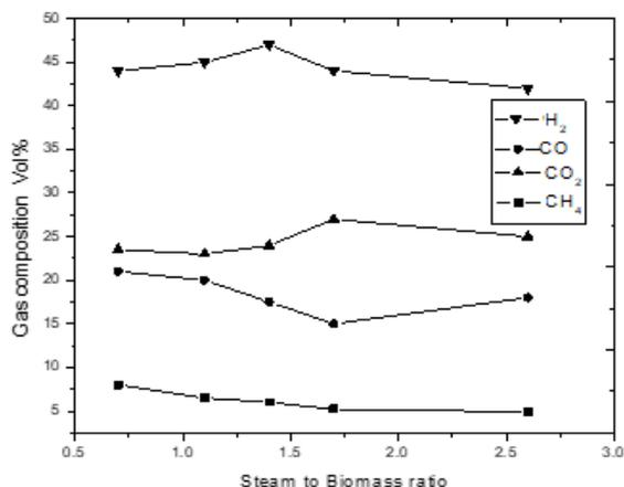
**Figure 7.** Influence of steam to biomass ratio on gas composition at a bed temperature of [710°C]
