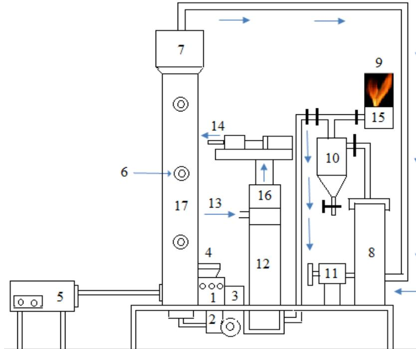
Figure 2. Fluidised Bed Gasification System – Experimental Setup
