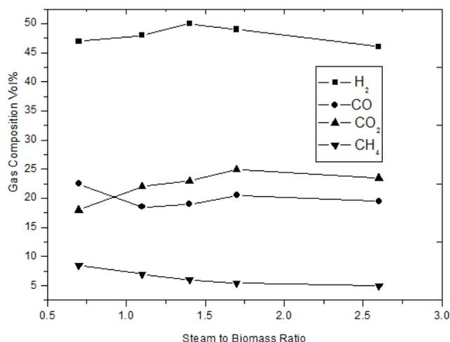
**Figure 8.** Influence of steam to biomass ratio on gas composition at a bed temperature of [780°C]
