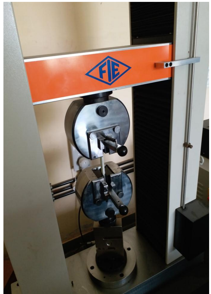
Figure 3. UTM Test Setup
