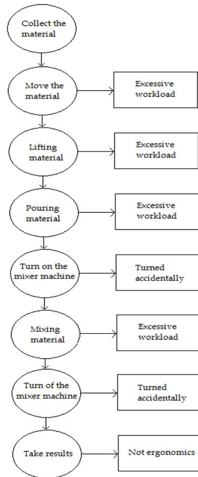
**Picture 4.** PFD of Mixing Process
