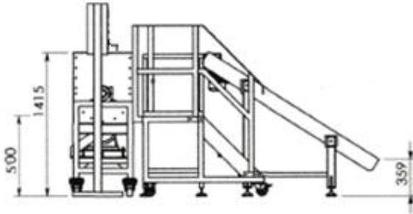
Picture 6. Side Dimension of Chosen Machine Concept
