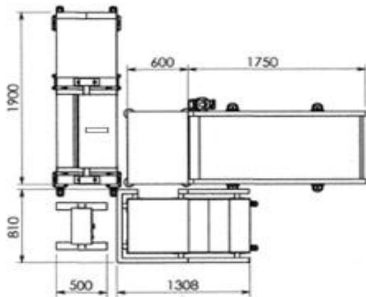
Picture 8. Top Dimension of Chosen Mixer Machine Concept
