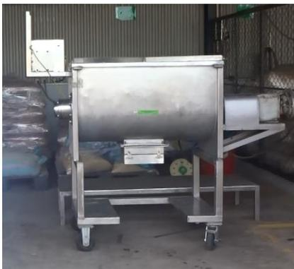
**Picture 1.** Current Mixer Machine for Waste Product
