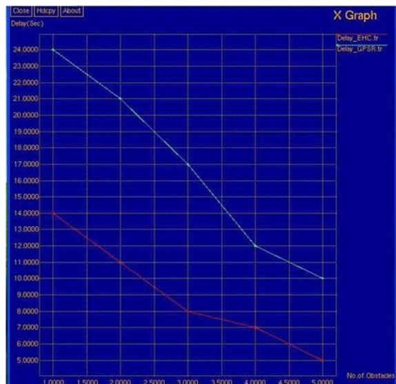
**Figure 15.** Comparison of Delay between EHC and GPSR
