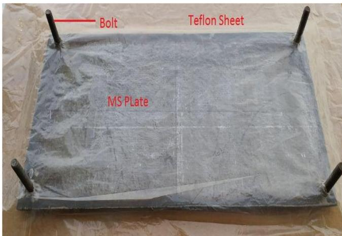
**Figure 2.** Mold for lamina
