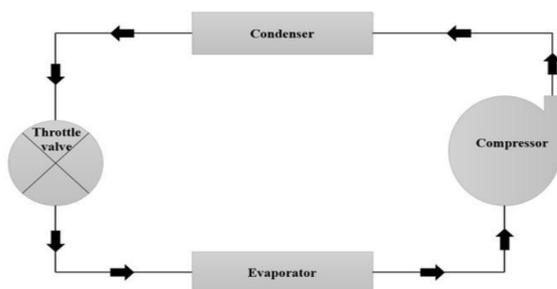
Figure 3 simple refrigeration cycle [11]
