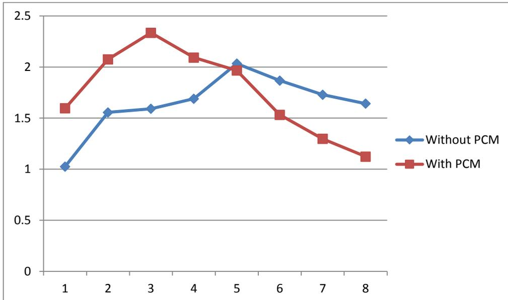
Figure 3. Comparison of COP at different load with and without CPM
