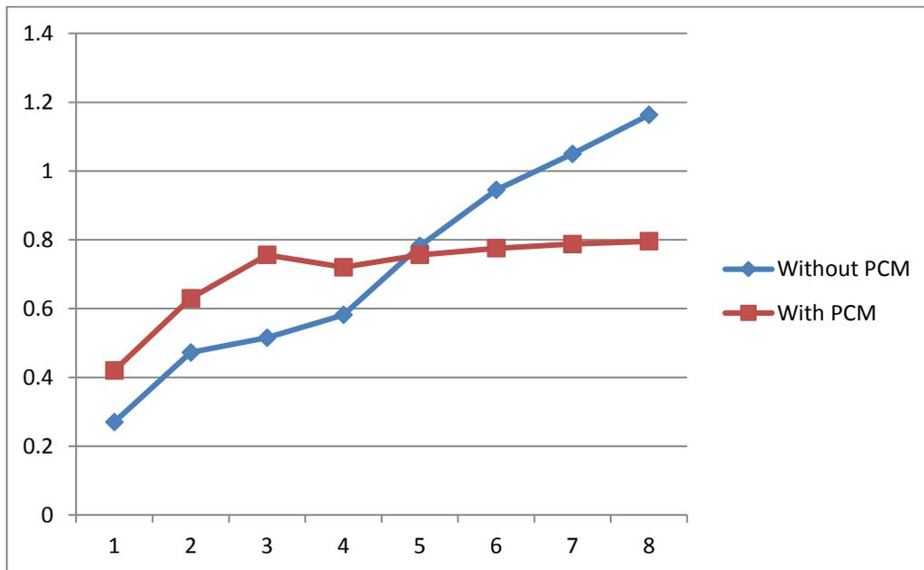
Figure 4. Comparison of Heat rejected at different load with and without PCM
