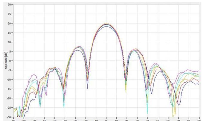
(a) Horizontal Antenna Beam Pattern
