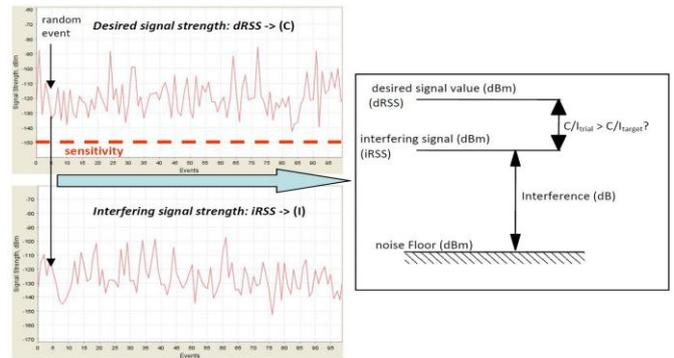
**Figure 3:** The criterion for evaluating interference
