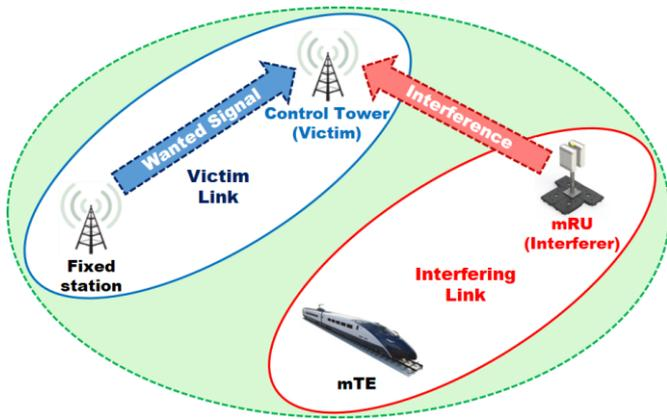
**Figure 1:** An interference Scenario between the Mobile radio Backhaul System and the Control Tower
