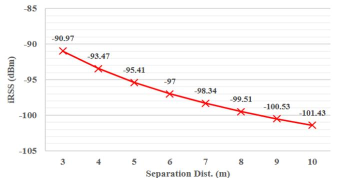
**Figure 4:** The iRSS in respect of the Separation distance
