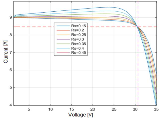
**Figure 3.** PV Simulation with different values of  $R_s$ .
