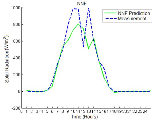
Figure 8. Comparison of measurement and prediction of solar radiation.
