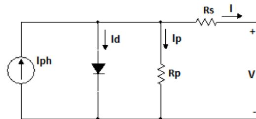
Figure 2. PV simplified Model.
