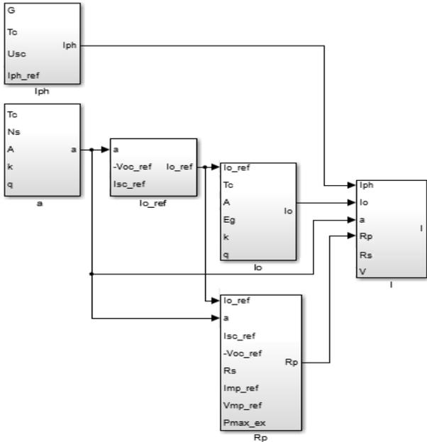
Figure 4. PV block diagram.
