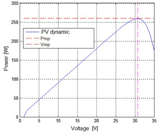
Figure 5. V-P Simulation using V-I values.
