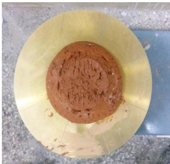
Figure 2: Table flow test of yellow loess mortar
