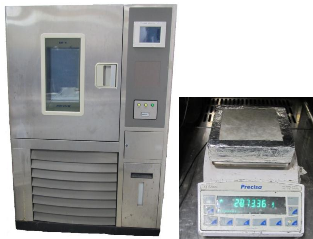
Figure 3: Humidity control Chamber and precision balance
