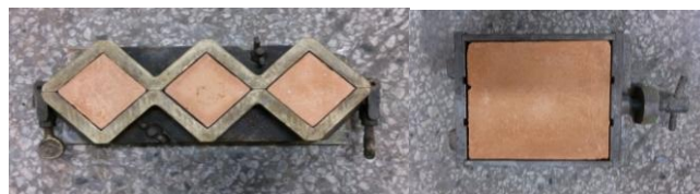
Figure 1: Yellow loess mortar specimen for compressive strength and moisture controlling experiment
