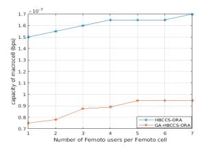
**Figure 6.** Capacity of macro-cell versus the number of femto users F in each femto-cell with the number of macro users M = 50
