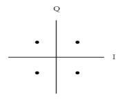
Figure 2. Constellation diagram for QPSK modulation.
