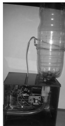
Figure 4. Connection between Arduino board, Wifi module and solenoid valve. Source: Authors
