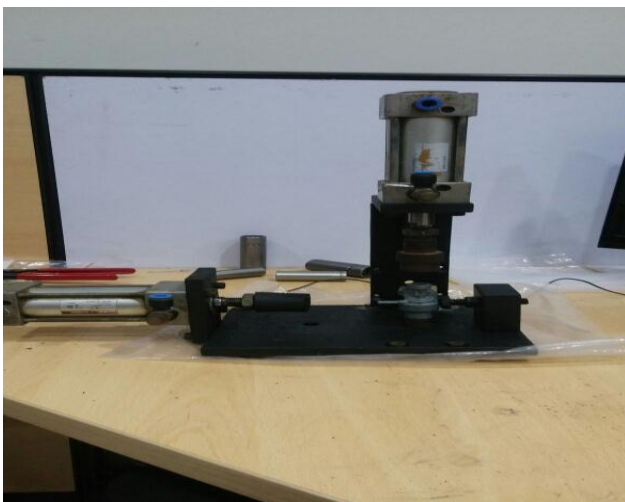
Figure 1. The mounted piston setup for sealing holes
