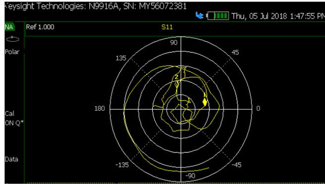
**Figure 1.9.** VNA Measured Result for partial ground structure
