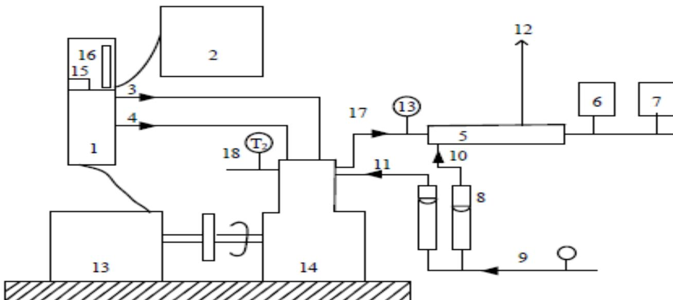
1-Control Panel, 2-Computer system, 3-Diesel flow line, 4-Air flow line, 5-Calorimeter, 6-Exhaust gas analyzer, 7-Smoke meter, 8-Rota meter, 9,11-Inlet water temperature, 10-Calorimeter inlet water temperature,12- Calorimeter outlet water temperature, 13- Dynamometer, 14-CI Engine, 15-Speed measurement,16-Burette for fuel measurement, 17-Exhaust gas outlet, 18-Outlet water temperature, T1- Inlet water temperature, T2-Outlet water temperature, T3-Exhaust gas temperature.
