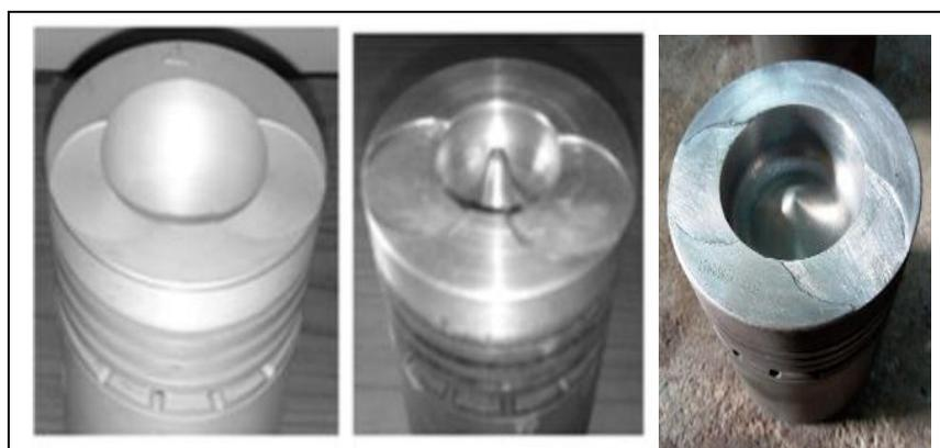
**Figure 2:** Hemispherical, Toroidal and shallow depth shapes
